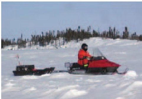
Dual channel GPR ice profiling equipment (being pulled behind a snowmobile) measuring ice thickness and water depth in a single pass
