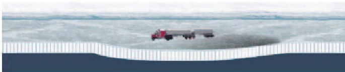
A slow-moving vehicle causes the ice to bend and forms a deflection bowl under the vehicle
