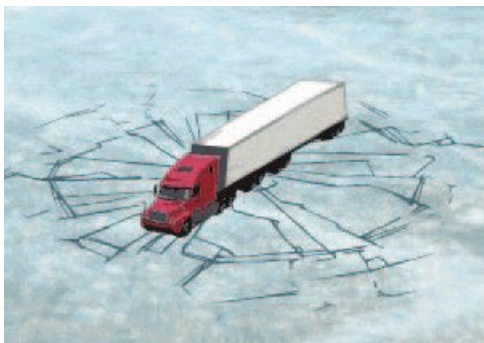
Plan view of radial (spoke-like) and circumferential (round) cracks forming on overloaded ice
